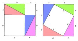
$b^2$ . When looking at the diagram on the right, the white area represents  $c^2$ . The large squares are identical. The space subtracted from them is identical. Therefore the remaining white space is identical and,  $a^2 + b^2 = c^2$ . The converse or opposite of the Pythagorean Theorem states that if in a triangle  $a^2 + b^2$  equals  $c^2$ , then the triangle is a right triangle. This is used when one has all of the sides of a triangle and wants to test if the triangle is a right triangle.
